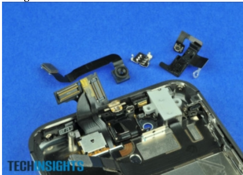
A closer look at the image sensors removed from the iPhone 4S.
