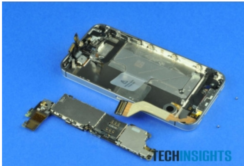
The main board removed from the iPhone 4S. This board is features a lot of shielding over the main components.
